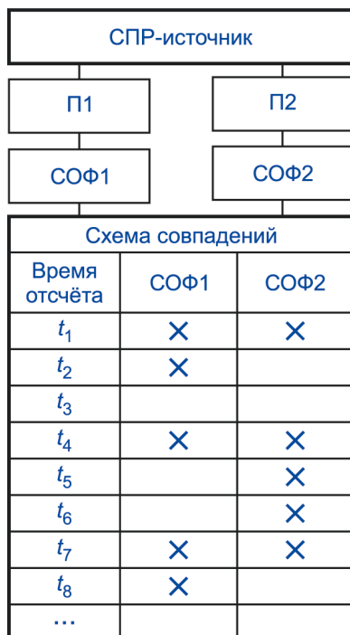
Fig. 2. The principle of operation of the coincidence scheme: SPD1, SPD2 – single photon detectors; the other symbols are the same as in fig. 1
